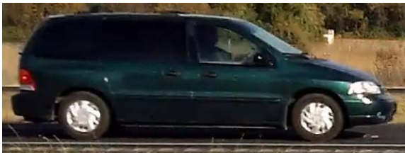
2002 Ford Windstar 16.8' Bumper-to-Bumper Length, 16.2' Video-Measured Length
