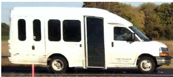
Van – Chev. Bus Hdcp 23.4' Bumper-to-Bumper Length, 21.0' Video-Measured Length
