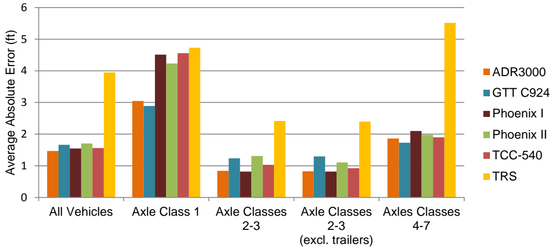
Figure 5.13: Average Absolute Error – Clustered by Axle Classification Grouping
