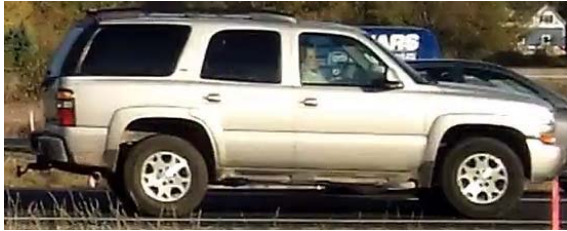
SUV – Full Size 2005-06 Tahoe 16.6' Bumper-to-Bumper Length, 16.2' Video-Measured Length
