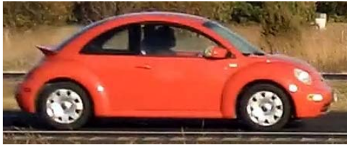
Auto – 2003-05 VW Beetle 13.4' Bumper-to-Bumper Length, 12.9' Video-Measured Length
