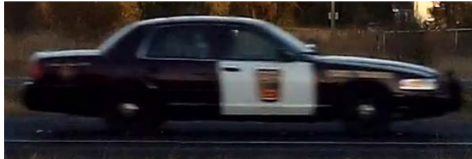
Auto – 2006 Ford Crown Victoria 17.7' Bumper-to-Bumper Length, 17.2' Video-Measured Length
