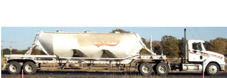
Semi – Bottom Dump Tank 56.8' Video-Measured Length
