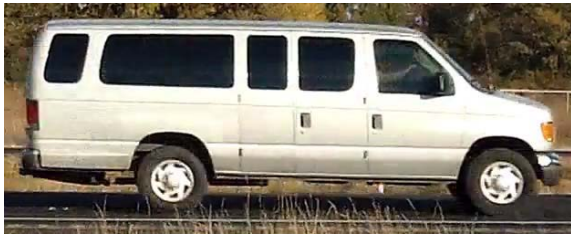
Van - Ford E350 18 Pass. 19.7' Bumper-to-Bumper Length, 18.6' Video-Measured Length
