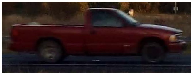
Pickup – 1994 Chev. S10 15.8' Bumper-to-Bumper Length, 15.3' Video-Measured Length
