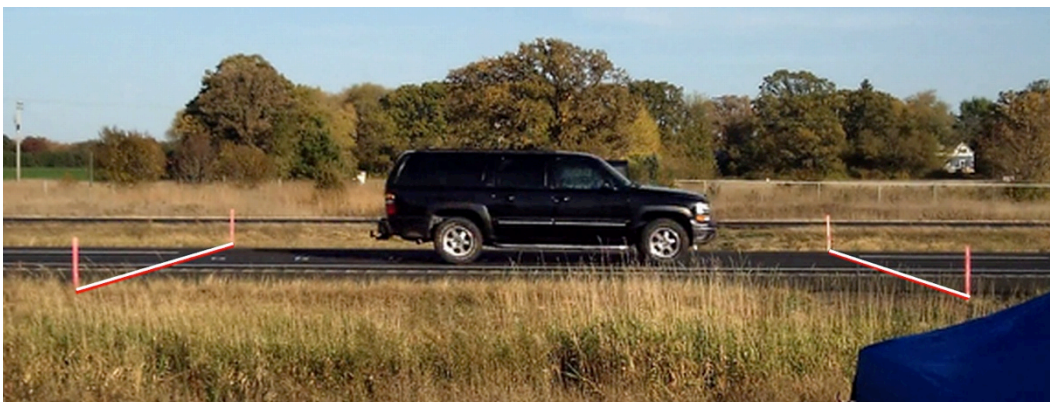
Figure 4.1: Field Test, Distance Marking Stakes (40-foot spacing on both sides)
